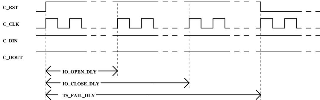
The figure below shows the timing for the deactivation sequence. As mentioned previously, these three delay times are not specified in either the ISO/IEC or EVM specification.
