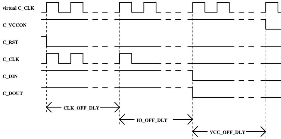
The figure below shows the timing for the Warm Reset sequence. The protocol state machine will not start a Warm Reset sequence until the reception of the character T0 (error-free) is complete.
