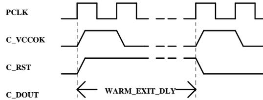
The figure below shows the timing of the C\_RST signal relative to the write that starts the Warm Reset sequence. This figure shows the earliest possible activation of the C\_RST signal. The exact delay depends on the C\_CLK divisor, because the C\_RST signal is synchronized to a rising edge on the C\_CLK signal.
