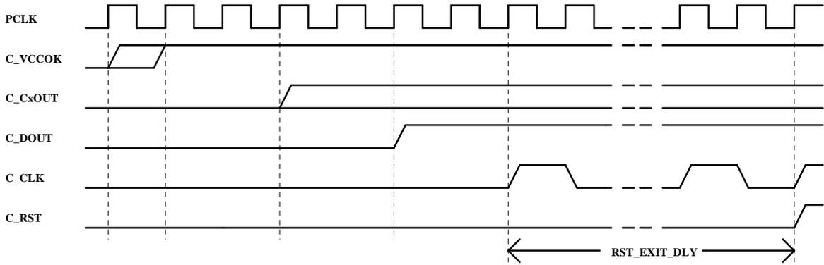
The figure below shows the timing of the C\_VCCON signal relative to the bus write that starts the card activation sequence. This write initializes the internal C\_CLK divider, for consistent timing.
