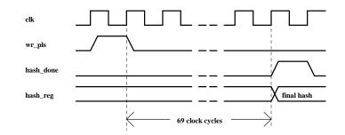
The figure below shows the timing for the last block of a message when the padding does require an additional block. If the FIFO is empty when this write occurs there will be an additional delay until the FIFO empty signal is deasserted. The number of clocks of delay to the deassertion of the **empty** signal is specific to the FIFO implementation.
