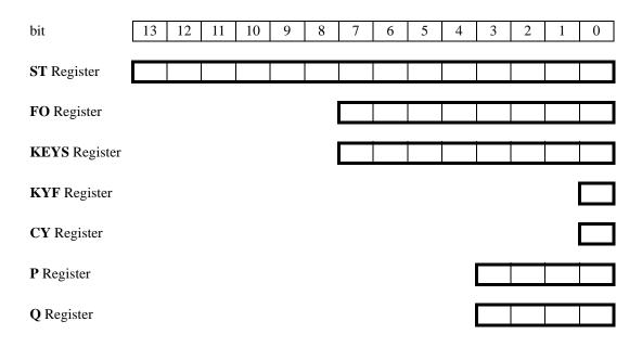
The P and Q registers are four-bit registers used to point to specific digits or ranges of digits in the general-purpose registers. When pointing to a specific digit only one of the registers is active at a time, but both are used when selecting a range of digits.
