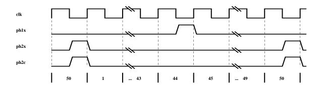
When running in one of the turbo modes, the external bus and ph2x are unaffected. However, the ph2c signal frequency is increased as shown in the figure below. Note that the ph2c signal is symmetric in all cases except for the 20x case.
