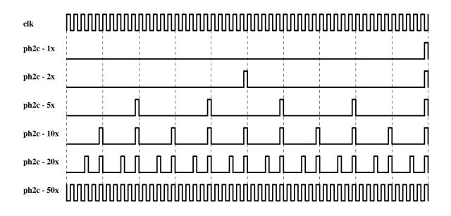
Both the external bus and the NEWT CPU operate with fixed machine cycles that are fifty-six clock (ph2x or ph2c) cycles long. These fifty-six clock cycles correspond to the fifty-six bits (or fourteen digits) of the Nut data word. The figure below shows a NEWT machine cycle.
