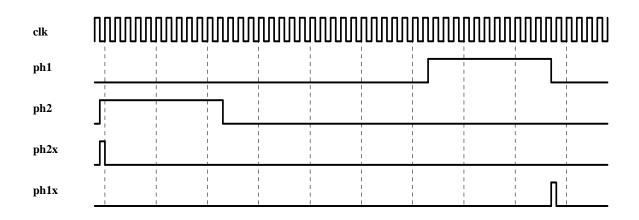
The ph1x and ph2x signals are used by the external bus portion of the design. A separate clock, called ph2c, is used by the logic of the CPU. When running in 1x mode ph2x and ph2c have the same timing. The details of this timing is shown in the figure below.
