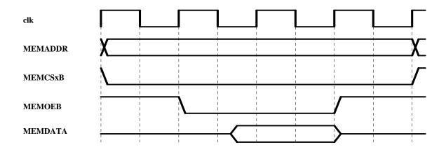
The timing for a memory write is shown in the figure below.
