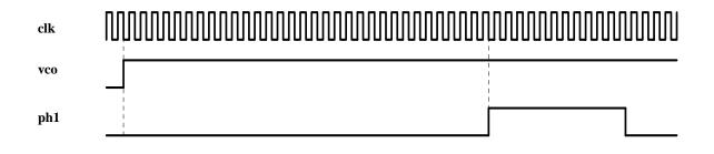
Even though the NEWT processor has begun operation at this point, the remainder of the system requires the **pwo** signal to be asserted to synchronize all system components to the NEWT machine cycle. These other components in the system require that the **pwo** signal change state at a specific time in the machine cycle, shown below.
