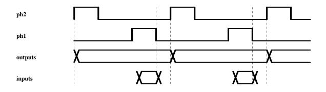
The NEWT CPU starts memory accesses of the physical memory at specific times during machine cycles, independent of the Turbo mode. Register accesses consist of four successive accesses. Note that register instructions are always executed in 1x mode, so all four physical memory accesses complete well before the end of the first bit time.
