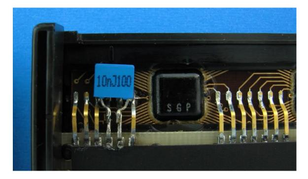
**7. STOP!** Before lifting the old CPU circuit board use a flashlight to look into the space between the CPU circuit board and the base circuit board. You will be able to see which type of connector is being used. The photo below shows the three types of connector used by HP.
