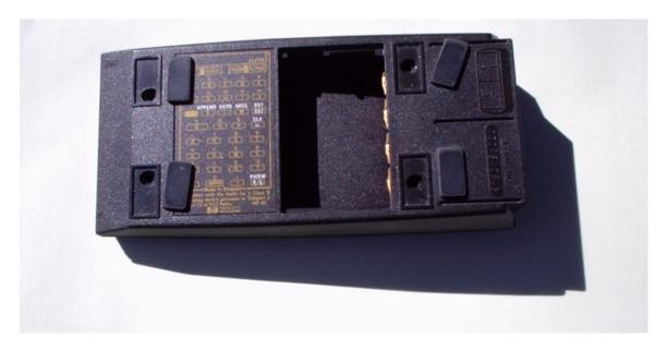
**6.** Lift off the bottom case and the U-shaped center case section. Note the orientation (front-to-back) of the center case section, because it not symmetric. Don't worry if your old CPU board looks slightly different from that shown in the picture below. These boards went through several revisions during the life of the 41C series.
