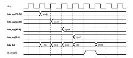
The diagram below shows a byte being written to the buffer, filling the buffer. The buffer is then emptied using four byte reads. Byte reads can have as little as one clock cycle between successive reads.
