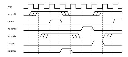
The tranmsit data out of the **endec\_top** module in the case of HDLC mode with an external clock uses the actual external transmit clock (**serx\_tclk**) to time the transmit data. However the decoder, in the same case, does not use the external clock to sample the receive data. This can be done externally to **hdlc\_top** if an edge-synchronous sampling point for the receive data is required.
