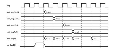
The diagram below shows word data being written to the buffer and rippling through before the first byte is taken by the transmitter.
