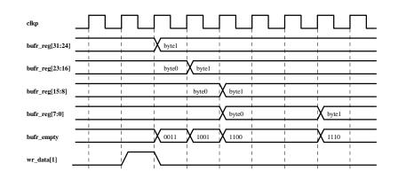
The diagram below shows long data being written to the buffer and then the first byte being taken by the transmitter.
