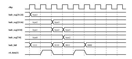
The diagram below shows a byte being written to the buffer, filling the buffer. The buffer is then emptied using a long read.
