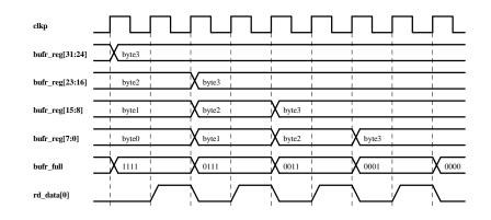
The diagram below shows a byte being written to the buffer, filling the buffer. The buffer is then emptied using two word reads. Word reads can have as little as one clock cycle between successive reads.
