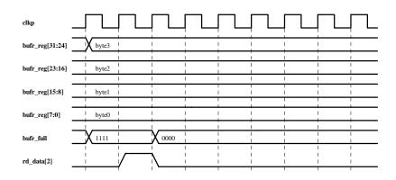
The diagram below shows the timing for the write of the last byte in an HDLC frame and the frame status update.
