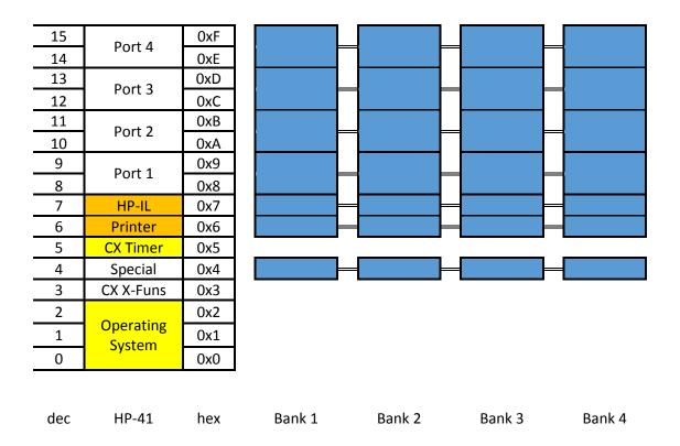
Every time the calculator is turned on software checks for collisions between physical modules and QROM, and disables any QROM blocks that would conflict with a hardware module. This collision check is only done for QROM blocks that are assigned to Bank 1. Collisions are not signaled in any way, because the user should be aware of what they plugged into the calculator.
