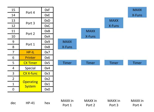
If the MAXX module is used in a 41CX the lower half of the Port where the module resides will be available for other uses, but the MAXX software always resides in the upper page of this Port.
